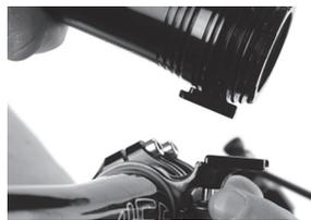
3. To release the light from the bracket pull down on the red button and gently pull back the light with your hand.
